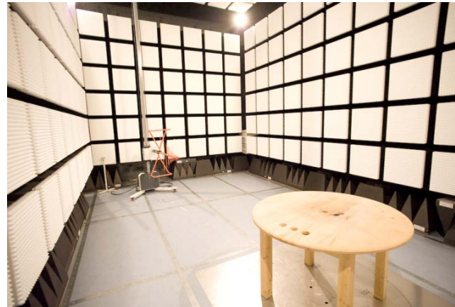
Semi-anechoic chamber for radiated RF measurements
