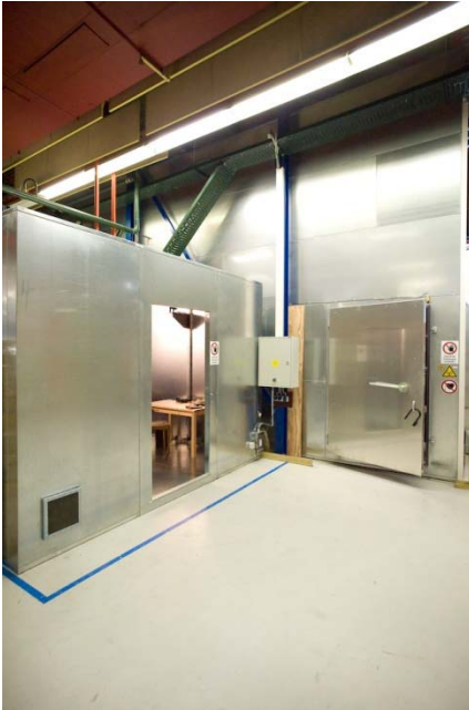
Shielded room for debugging and conducted RF measurements
